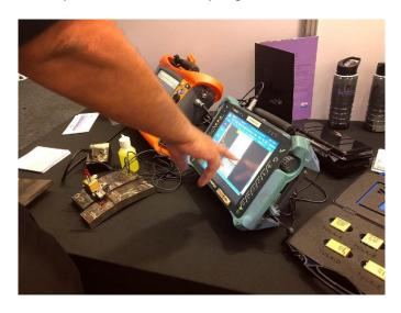
TULA™'s concept has also been applied to angle beam probes for the purpose of detecting HTHA in weld HAZ regions.
